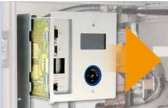
1. Control electronics are easy to remove.
